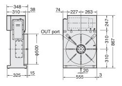
Rotary joint shown in layout is optional. In ports are located in back side.
