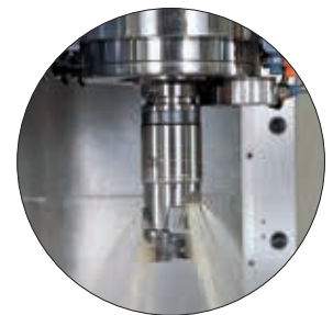
High Pressure Coolant Through Tool
