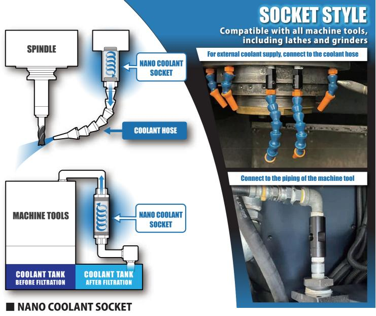
The nanocoolant socket, which incorporates a built-in nanocoolant generator, can be attached to coolant hoses or piping. It enables machining with external lubrication and can be widely used on machine tools other than machining centers, such as lathes and grinding machines.
