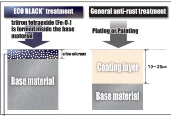
The surface part that has become a porous structure by the black rust is treated with a water displacer by plant-based rust preventive oil, which replaces the moisture and oil in the pores. As a result, a more advanced rust prevention treatment is achieved.
