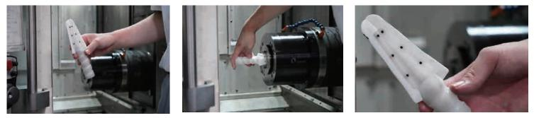
NIKKEN Silicone Taper Scraper capable of surely and quickly performing regular maintenance of a machine spindle bore taper.
