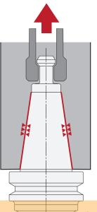
The condition of the taper connection is one of the most important factor for the machining operation.
