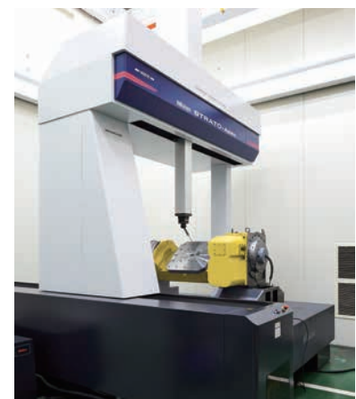
Accuracy measurement with large 3 Dimensional Measuring Machine
