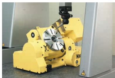
5AX-230 on 3 Dimensional Measuring Machine
