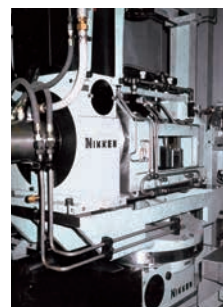
CNC401T is installed on CNC600.
