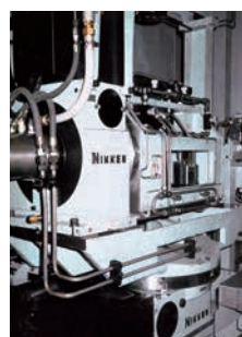
CNC401T is installed on CNC600.
