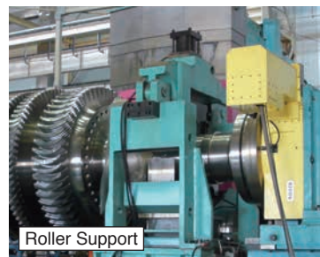
CNC1201 Indexing of the turbine shaft. Turbine shaft is supported and clamped by the roller support.
