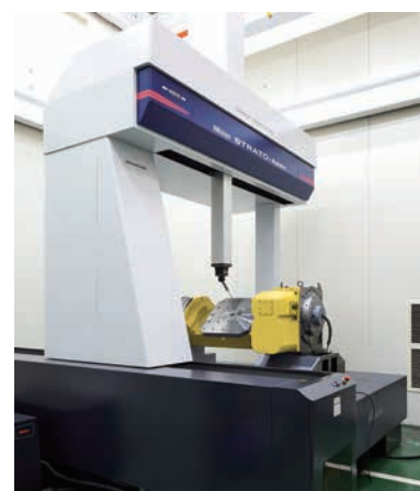
Accuracy measurement with large 3 Dimensional Measuring Machine
